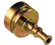
Steel valve piston with a T.I.R. of .005", a 32 micro seat and 50 micro for the "O"-ring grooves
